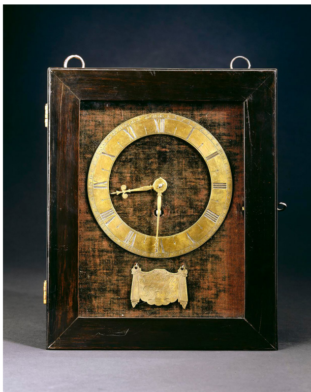
Haagsche Klokje (1657-1659) by Salomon Coster. This is one of the earliest pendulum clocks ever made following Christiaan Huygens's design of 1656. Photo courtesy the Science Museum, London
