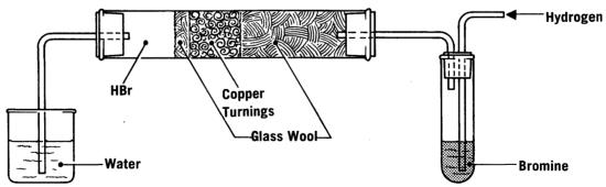
Hydrogen is bubbled through the bromine after the air has been driven out of the apparatus. The mixture of the two gases is passed over heated glass wool, where combination takes place. Copper is used to remove any uncombined bromine. The gas is bubbled through water to form a solution of HBr.
